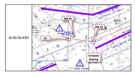
Figure 23 – Illustration of compass bearing between KS and JDR 19
