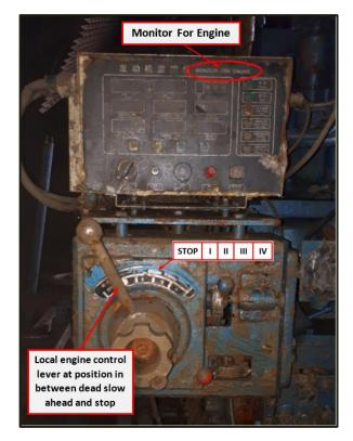
Figure 18 – Engine local control lever at position between Dead Slow Ahead and Stop, photo taken in the engine room after vessel was salvaged
