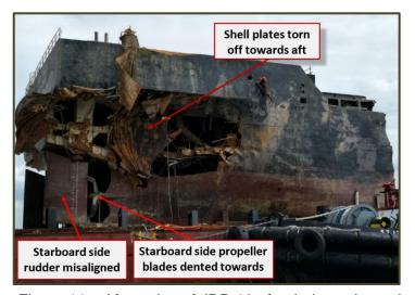
Figure 11 – Aft section of JDR 19 after being salvaged
