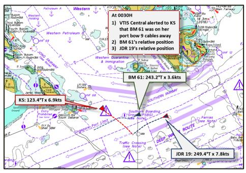
Figure 5 - Relative position of BM 61 and JDR 19 to KS, at 0030H
