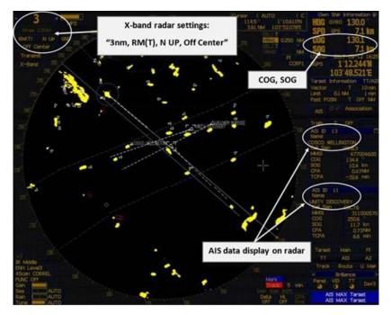
Figure 14 – X-band ARPA display setting on KS before crossing the TSS
