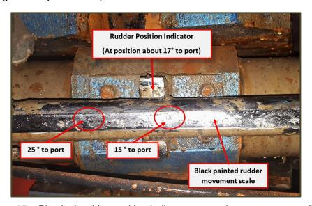
Figure 17 – Physical rudder position indicator at steering gear room on JDR 19
