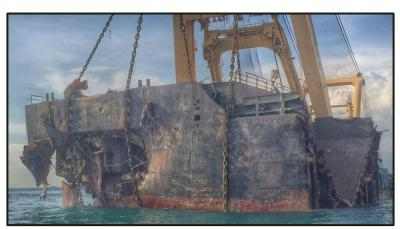
Figure 9 - The starboard quarter of JDR 19 being lifted out of water showing the angle and location of impact from KS's bow.
