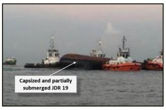
Figure 8 - Capsized and partially submerged JDR 19 was towed by four tugs (Source: Maritime and Port Authority of Singapore)
