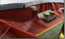
Figure 10 – Damage at ship bow areas after the collision (Source: the ship's manager)
