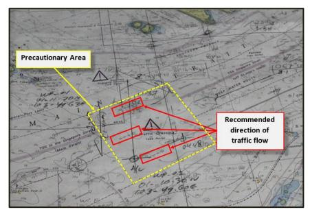
Figure 20 – BA 4041 used by KS overlaid with annotations indicating recommended direction of traffic flow within the Precautionary Area
