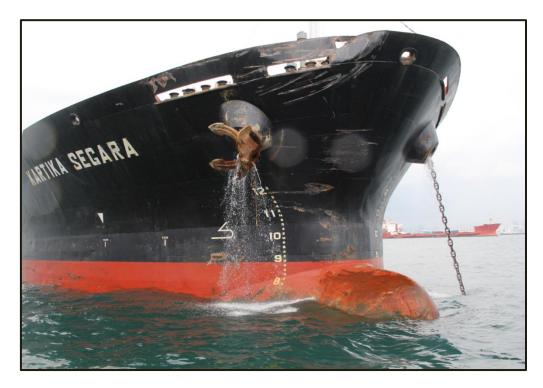
Figure 1: Kartika Segara – Photograph after collision showing damaged bow
